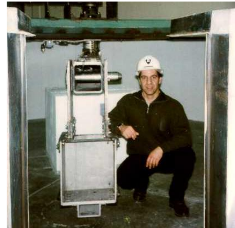
Mine centrifuge used to generate high g-forces to model mining problems.
