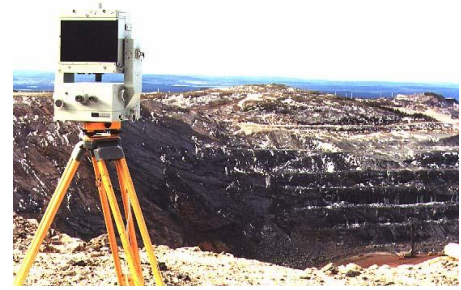
Pit wall stability being automatically monitored by computer controlled laser survey instruments.
